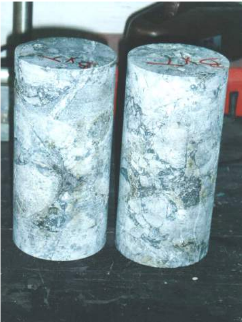
Fig. 20. 100 mm diameter by 200 mm long specimens of Braden Breccia from the El Teniente mine in Chile
